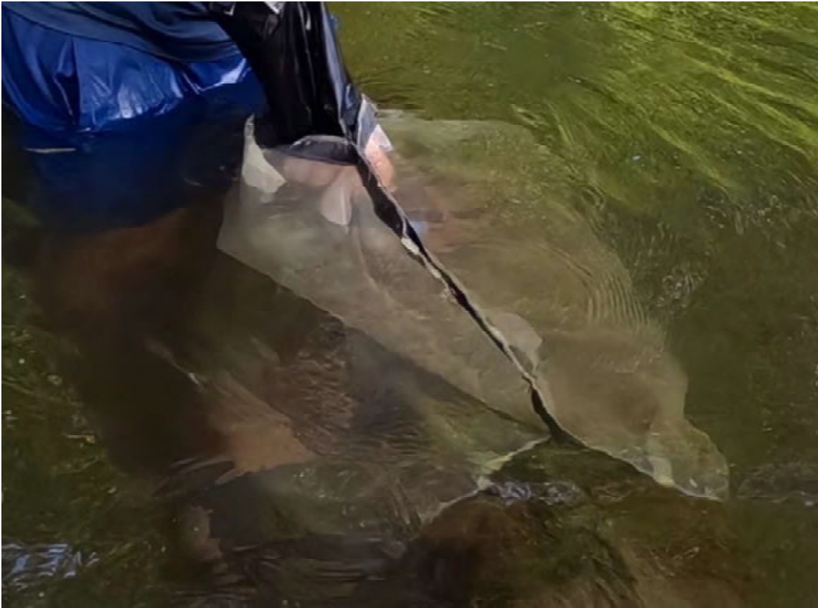
Figure 5: Using the snag bag to sample macroinvertebrates in the Peel River. Arm reaches in through the black sleeve at top of picture to scrub the snag inside the snag bag.
