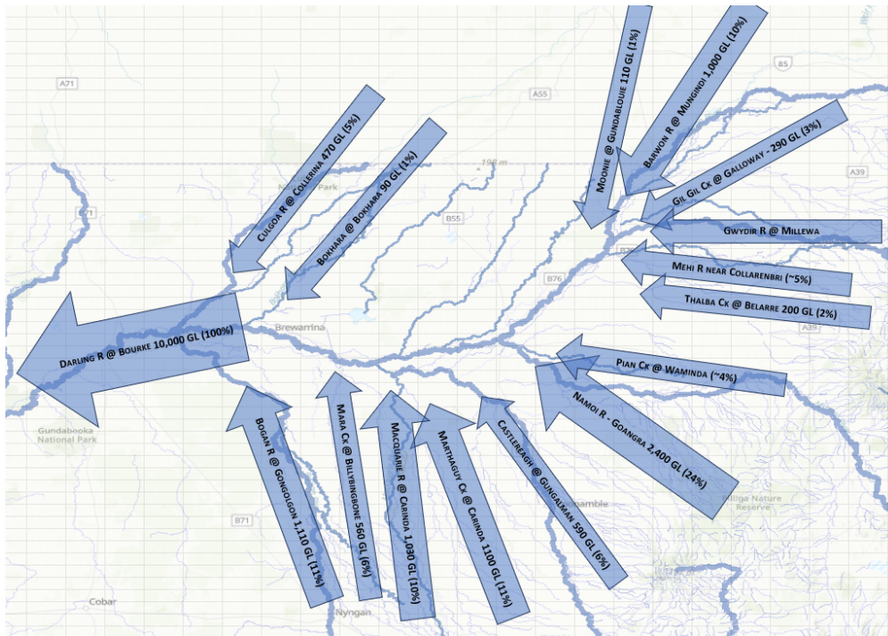
Figure 24. Summary of total main river and tributary flow volumes, Mungindi to Bourke, September 2022 to January 2023
